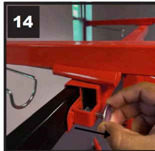
14. To extend the outriggers for use, pull out on the outrigger lock pin with your right hand and slide the outrigger out with your left hand.
