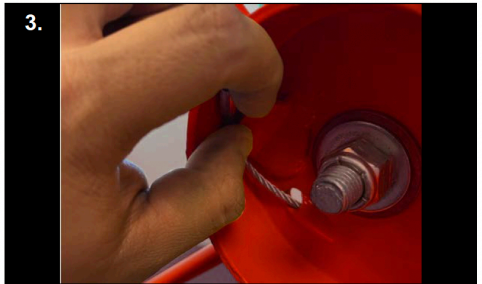
3. Pinch and pull the cable out from the winch drum. BE CAREFUL! a worn cable can have frayed strands. Wearing gloves will help protect your hands.
