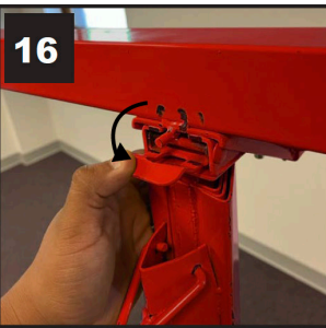
16. Flip out the tilt latch to allow the cradle to tilt for loading and for hanging drywall on sidewalls and sloped ceilings.
