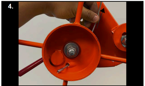
4. Once the cable tab is pulled out from the mooring tab, then pull the cable out of the winch drum hole.
