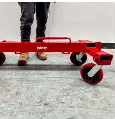
6. With the arms stowed and locked in the storage and transport position, the cart can be conveniently handled for compact transportation.
